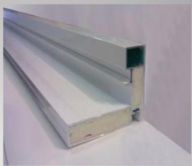
**Door frame** in extruded aluminum Made of L-shaped extruded aluminum with double thermal break, treated 20-micron anodizing or white lacquared.
